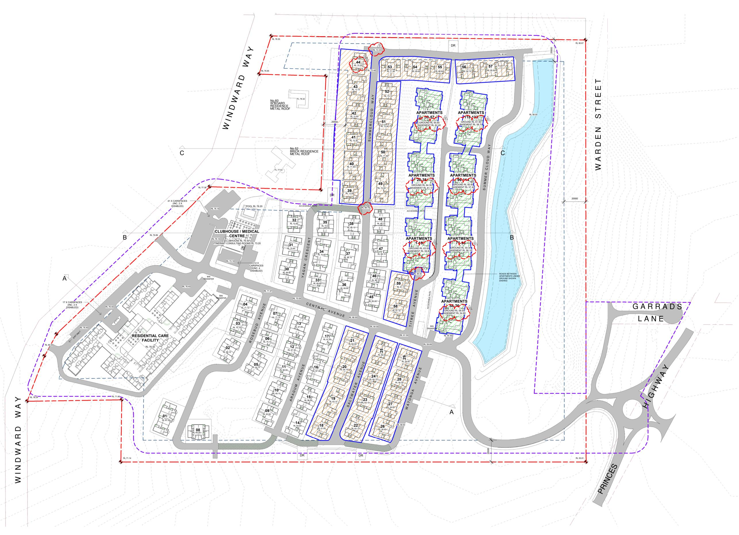
STAGE 1 - RCF, CLUBHOUSE & 26 X DUPLEX, 4 X TRIPLEX INCL SITE CIVILWORKS OVER ALL STAGES STAGE 2 - 24 X DUPLEX, 5 X TRIPLEX STAGE 3 - APARTMENTS
